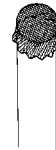
If the wire screen breaks or comes off the pipe, replace it at once.
